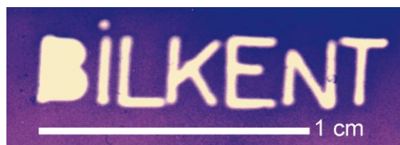
Fig. 2. Photograph of macro-scale lithographic example of PVC film containing methyl violet (10:1 by weight).
